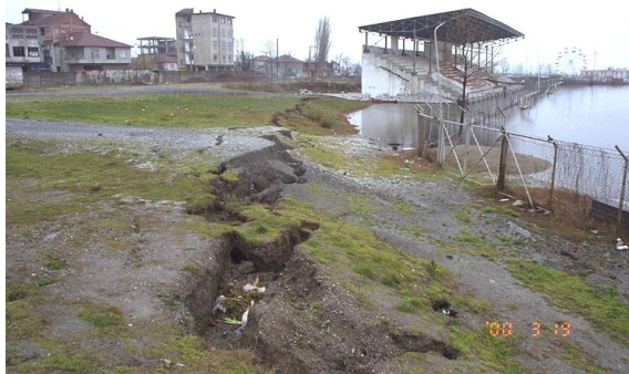
Photo 2.3.5. Fault rupture and submerged field in Kavakli district, Golcuk, Mar. 2000 (Refer to color Photo 11).
