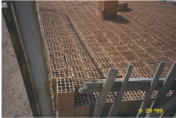
Photo 2.2.5. Hollow clay block for infill wall, Yalova (Refer to color Photo 3).
