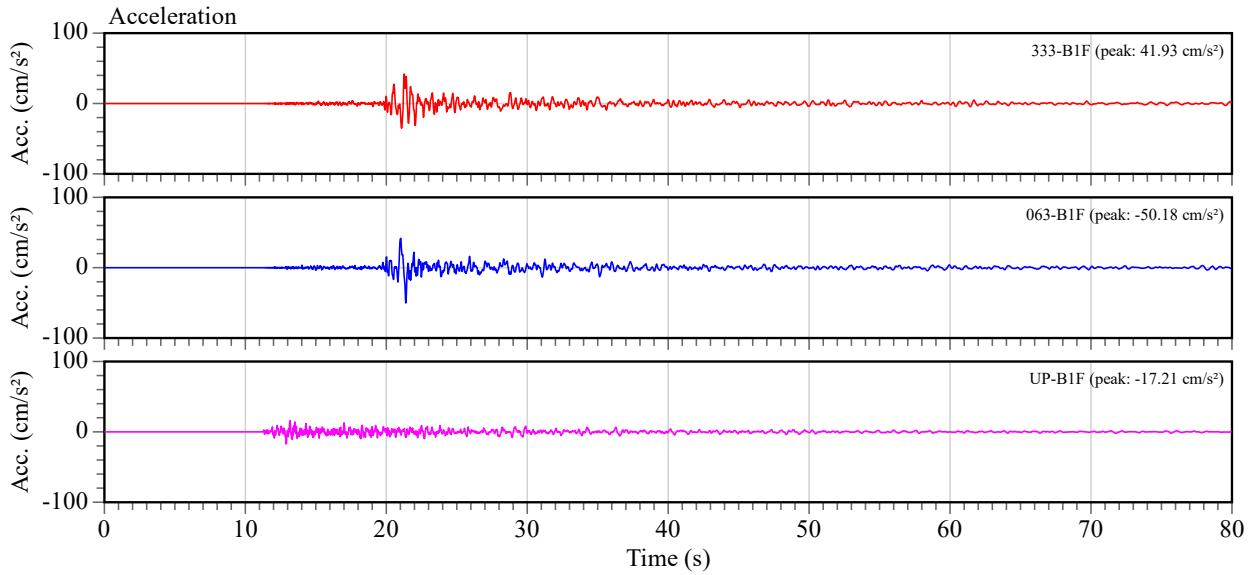
Fig. 2.1 Acceleration waveforms of B1F at the station CHPM
